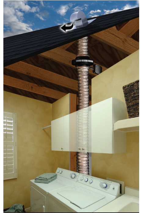
NOTE The PV-100x Dryer Booster fan is suitable for use with duct runs of up to 105 linear feet of 4" rigid duct or a maximum of 6 elbows and 80 feet.
